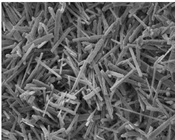
Figure 6. Moonmilk from Rock-me Cave (TR52), Timor, NSW. The thickest fibre in this photo is \approx 2\mu\text{m} (0.002 mm) wide. The sample only contains calcite fibres. Image by Brian England
