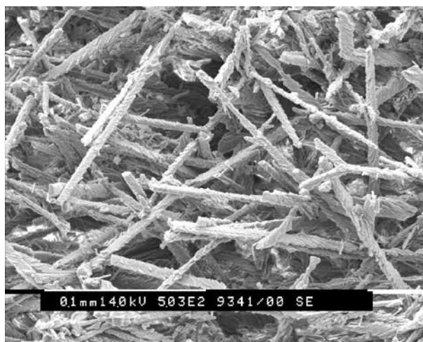
Figure 5. Moonmilk from B4, Kunderang Brook, NSW. Calcium carbonate strands are approx. 7.08\mu\text{m} (0.00708 mm) thick. Image by Brian England
