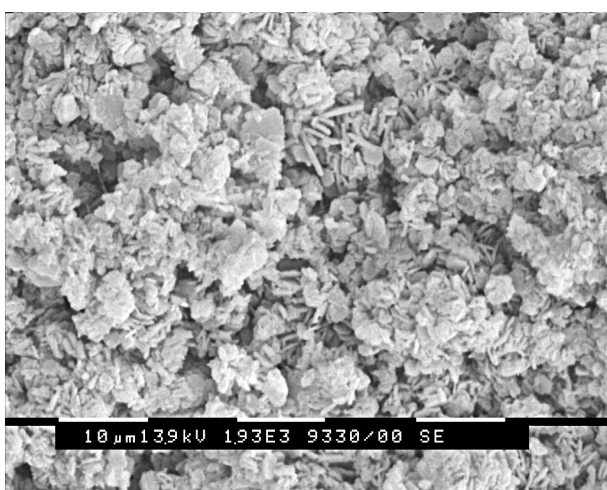
Figure 8. Moonmilk from Wiburds Lake Cave (J58), Jenolan NSW. White section on scale bar is 2\mu\text{m} (0.002 mm) long. Image by Brian England
