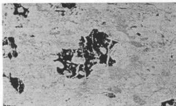
Figure 3 Pyrite in palaeokarst breccia, Lune River Quarry, Tasmania. Thin section. Transmitted light. Crossed nicols. Pyrite forms opaque masses around large original clasts. Long axis of central pyrite mass is 5 mm.
