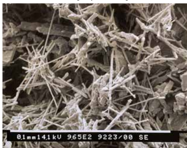
Figure 11. Moonmilk from Mammoth Cave (J13) Jenolan NSW. Sample contained both calcite and aragonite. Fibrous calcite strands are approximately 1.5\mu\text{m} thick. Image by Brian England
